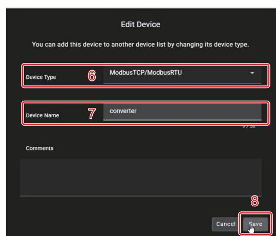
The previously scanned IP address and **converter** will now appear under the **ModbusTCP/ModbusRTU** field.
