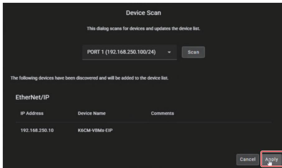
You will return to the *Device List Screen*. Confirm that the devices have been updated. In this example, **K6CM-VBMx-EIP** is added to **Ethernet/IP**.
